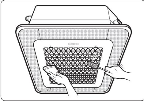
Wipe the surface of the unit with a slightly wet or dry cloth when needed. Wipe off dirt of odd-shaped areas by using a soft brush.
