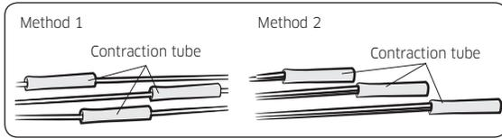
6 Wrap it with the insulation tape twice or more and position your contraction tube in the middle of the insulation tape.
