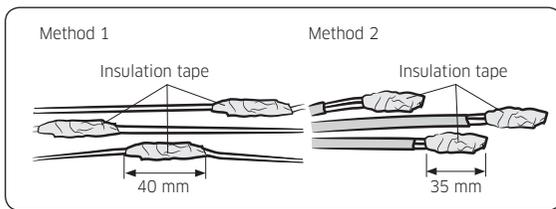
7 After tube contraction work is completed, wrap it with the insulation tape to finish. Three or more layers of insulation are required.
