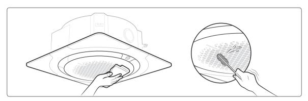
Wipe the surface of the unit with a slightly wet or dry cloth when needed. Wipe off dirt from odd-shaped areas by using a soft brush.
