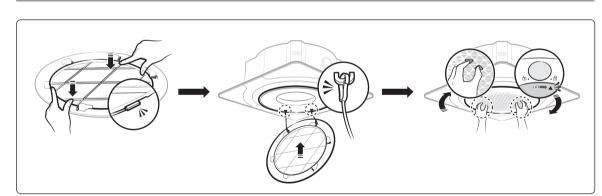
After cleaning and reassembling the air filter, reset the filter-cleaning reminder as follows:
