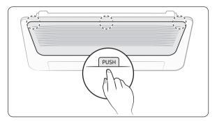
Press the **Push** signs on the front panel, then open the grille.
