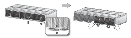
2. Clean the Air filter with a vacuum cleaner or soft brush. If dust is too heavy, then rinse it with running water and dry it in a ventilated area.
