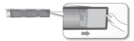
2. Clean the Air filter with a vacuum cleaner or soft brush. If dust is too heavy, then rinse it with running water and dry it in a ventilated area.
