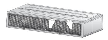
2. Clean the Air filter with a vacuum cleaner or soft brush. If dust is too heavy, then rinse it with running water and dry it in a ventilated area.
