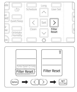
After cleaning and reassembling the air filter, be sure to reset the filter-cleaning reminder as follows:
