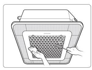
Wipe the surface of the unit with a slightly wet or dry cloth when needed. Wipe off dirt of oddshaped areas by using a soft brush.
