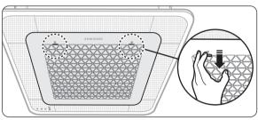
Push down the hooks at each side of the front grille to open the grille.
