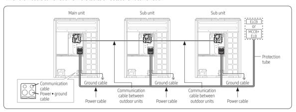
\* Power Supply cords of parts of appliances for outdoor use shall not be lighter than polychloroprene sheathed flexible cord. (Code designation IEC:60245 IEC 66 / CENELEC: H07RN-F)
