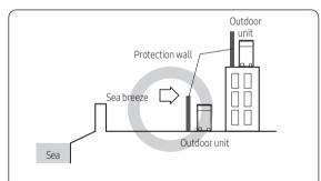
Protection wall should be constructed with a solid material that can block the sea breeze and the height and width of the wall should be 1.5 times larger than the size of the outdoor unit. (You must secure more than 700mm of space between the protection wall and the outdoor unit for air circulation.)
