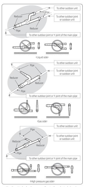
\* Use the attached reducer according to the selected pipe size.
