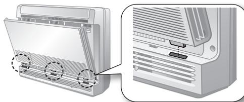
2. Grab the handle and slightly press the air filter down to bent the air filter. Then, pull the Air filter towards you and lift it up to remove the Air filter.
