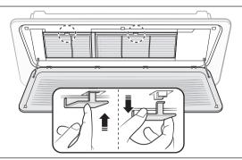
Pull the air filter out of the indoor unit
