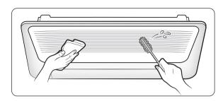
Wipe the surface of the indoor unit with a tepid damp cloth.
