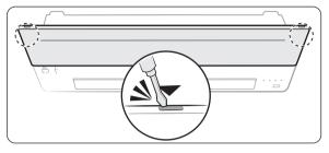
Insert a driver at the marked points and open the front grille.
