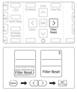
After cleaning and reassembling the air filter, be sure to reset the filter-cleaning reminder as follows:
