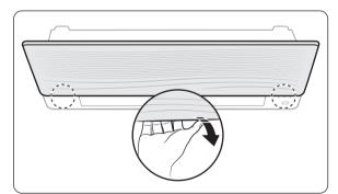
Insert your hand into the front grille and pull out the front grille to open it.
