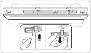
Press the **Push** signs on the air filter. Grab the handle of the air filter and pull it out from the indoor unit.
