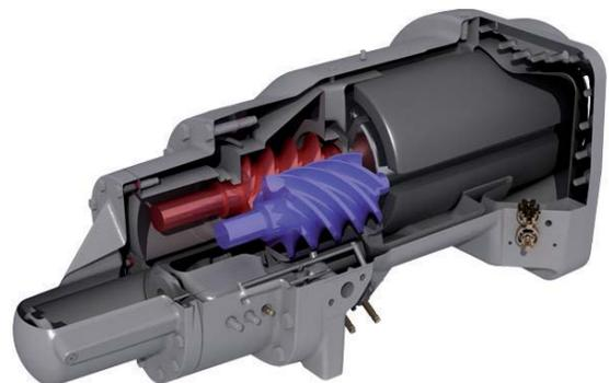
The compressor is driven by a high-efficiency motor optimized for water-cooled chiller operation. The rotors feature the latest lobe design for R134a operation, running in oversized roller bearings and with variable slide valve capacity control.
