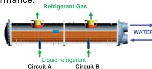
The external and internal tube surfaces are micro-grooved, resulting in an increased surface area and enhanced heat transfer.
