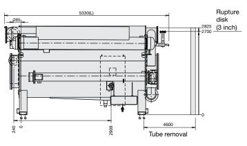
NOTE: Dimensions are for guidance only. Refer to the certified drawings supplied upon request when designing an installation.
