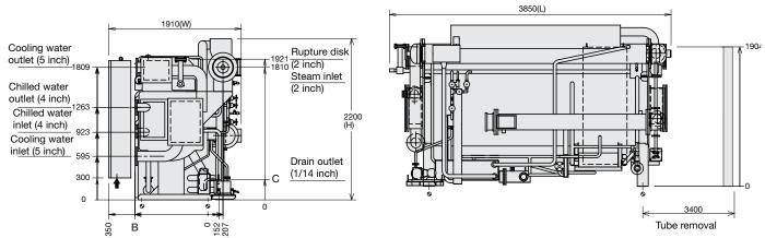
NOTE: Dimensions are for guidance only. Refer to the certified drawings supplied upon request when designing an installation.
