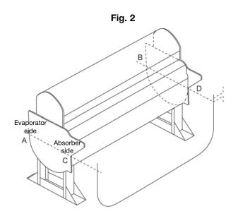
• If tolerances are not met, shim the appropriate points by inserting a metal spacer between the machine base and the foundation. The metal spacer size is approximately 50 mm wide by 80 mm long. Prepare spacers with different thicknesses (0.6 mm to 9 mm).
