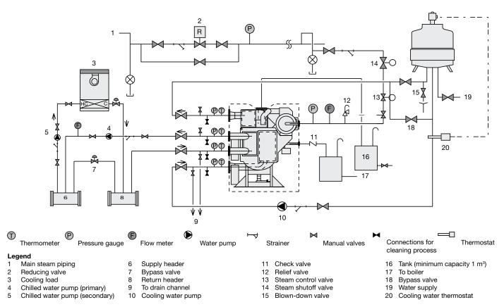
NOTE: In order to prevent freezing of the chilled water during the chiller dilution cycle, ensure continued operation of the chilled water pumps and cooling load until the dilution symbol on the control panel goes off. For the same reason the chilled water volume must be higher than 10.5 litres/kW.
