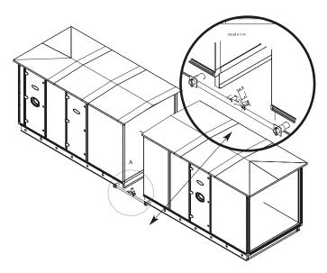
Place the casing sections as close as possible together before assembly. Pull the casing sections towards each other by placing the lifting bars first in one and then in the other casing section. Then pull both parts towards each other using pull ropes.
