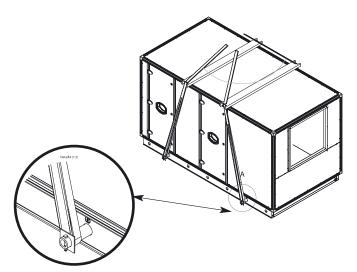
The AHU should not be lifted or moved under the cross beams. This is indicated by the label below.
