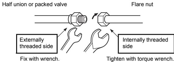
2. As shown in the figure, be sure to use two wrenches to loosen or tighten the flare nut of the valve on the gas side. If you use a single crescent, the flare nut cannot be tightened to the required tightening torque.
