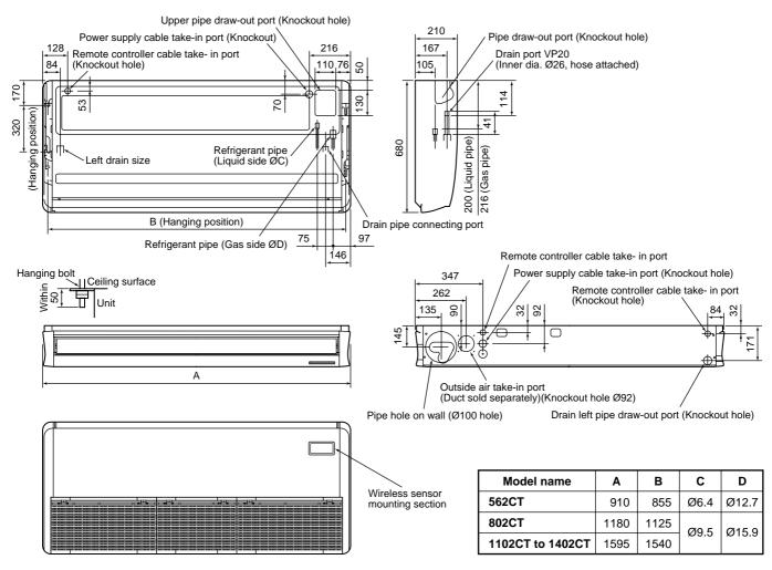
Considering pipe/wire connecting work inside the ceiling after the indoor unit has been hanged, select an installation place and determine piping direction.
