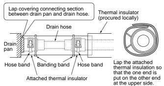
\* Tighten the banding band so that attached thermal insulator is not pushed excessively.
