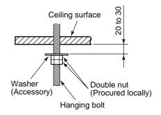
2) Hang the unit to the hanging bolt as shown the figure below.
