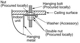
\* Tighten the hanging metal with upper/lower nuts as shown in the figure.
