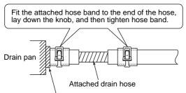
Confirm that soft hose is pushed in up to the end of the drain pan.
