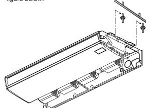
3) As shown in the figure below, fix the ceiling material securely with the double nuts.
