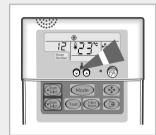
4 Select the fan speed by pressing the Fan button one or more times until the intended value is displayed :
