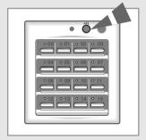
2 In order to turn ON/OFF a specific air conditioner connected to the centralized controller, press the (Specific ON/OFF) button.
