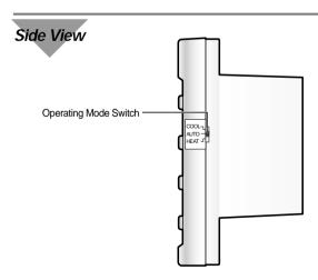
Mole ◆ Choose the appropriate operating mode with the Operating Mode Switch that enables the user to choose between the Cool/Auto/Heat mode.
