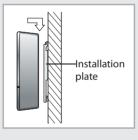
**3** Hang the DMS2 on the groove which is on the top of the installation plate.
