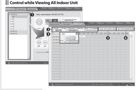
Total Control menu is a menu to view all status (Operation On/Off, Peak Control, Error Status, Assign indoor unit or not) of connected indoor units at a look. Also, users can set the Remote Control Setup and the Upper & Lower Temperature Setup for all indoor units.
