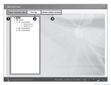
This is a function to inquire the physical connection status and error status for indoor units and outdoor units that form the DVM system, detailed information of indoor units and outdoor units.
