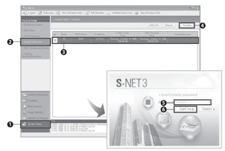
This function creates new device information when a device has been added or edited. The tracking process takes about 5 minutes.
