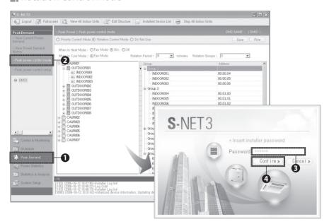
Different groups of indoor units can be selected for peak power management This function allows you to set the rotation level for each indoor units.
