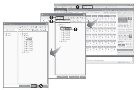
This function allows you to organize air conditioners into a structure that is easier to manage, regardless of the actual installation structure. You can divide the entire air conditioning system into different zones by creating new zones.
