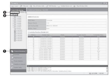
This function allows you to monitor the status of DMS and the status of centralized controller, peak controller and power interface module connected to the DMS.
