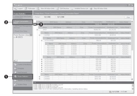
This function allows you to check the distributed results of power consumption and rated bill in power management structure or management structure.
