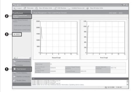
This function allows you to check the control status of the current power demand controller real-time by each DMS.
