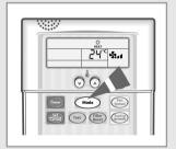
2 To select the HEAT mode, press the Mode button until is is displayed at the top of the wired remote controller.
