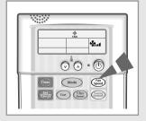
3 Select the fan speed by pressing the (speed) button one or more times until the intended value is displayed:
