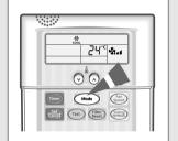
2 To select the COOL mode, press the houton until is displayed at the top of the wired remote controller.
