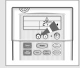
4 Select the fan speed by pressing the (speed) button one or more times until the intended value is displayed:
