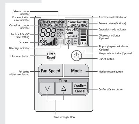
When controlling multiple ventilators with one ERV wired remote control, the ERV wired remote control displays the status of one random ventilator only. If multiple ventilators are controlled by one ERV wired remote control only and an external controller is used to control one of the multiple ventilators, the ERV wired remote control will display the status of the randomly selected ventilator and it may differ from the status of some other ventilators.
