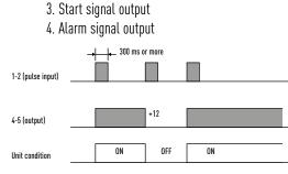
NOTE: The wire length from indoor unit to the Relay must be within 2.0 m. Pulse signal changeable to static with JP cutting. (Refer to JP001)
