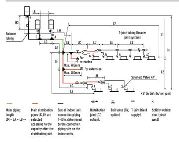
The outdoor connection main tubing (LO portion) is determined by the total capacity of the outdoor units that are connected to the tube end Note: Do not use commercial T-pieces for the liquid pipes of the distribution joint.
