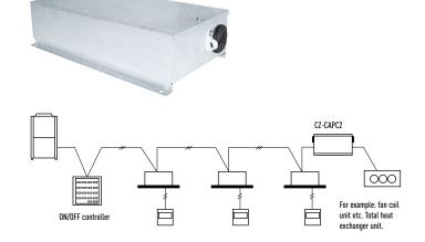
· Control and status monitoring is possible for individual indoor unit (or any external
