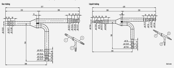
CZ-P1350PH2BM: For outdoor unit side (Capacity after distribution joint is greater than 68,0kW and no more than 168,0kW).
