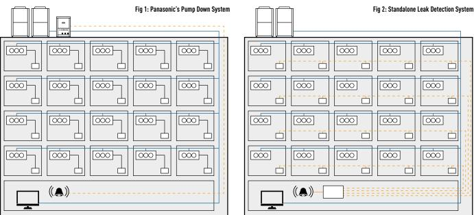
Due to the simplistic installation and control interfacing, shown in Fig 1, Panasonic's ECOI Pump Down System can provide dramatic reduction in capital cost and installation time when compared to a standalone leak detection system, shown in Fig 2. This option is ideal for hotels, offices and public buildings where safety of building occupiers is a must and is extremely cost effective, savings of 40% can be easily achieved.
