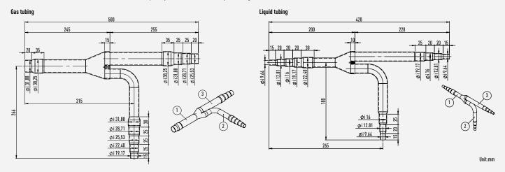
CZ-P224BK2BM: For indoor unit side (Capacity after distribution joint is 22,4kW or less).
