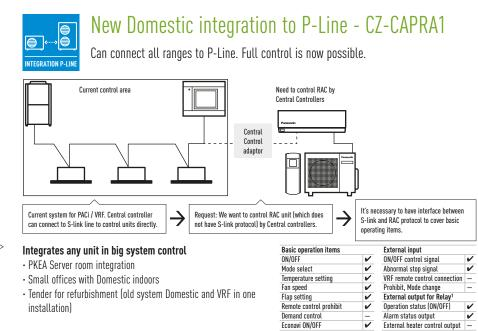
1) Because current CN-CNT connector can not provide the power for external output relay, additional power input for external relay is necessary.
