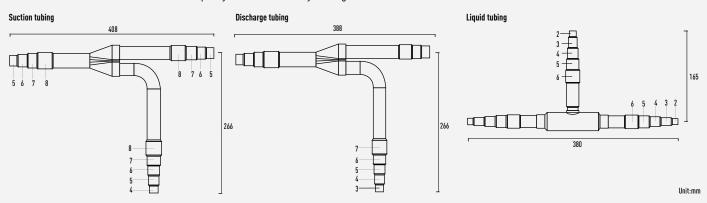
CZ-P680BH2BM: For outdoor unit side (Capacity after distribution joint is greater than 22,4kW and no more than 68,0kW).
