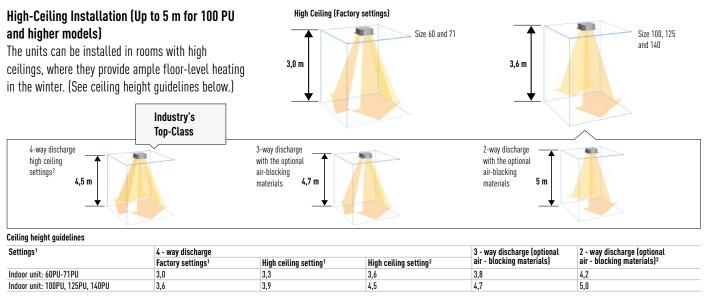
1) When using the unit in a configuration other than the factory settings, it is necessary to make settings on site to increase airflow. 2) Use air-blocking materials (CZ-CFU2) to completely block two discharge outlets for 2-way airflow.
