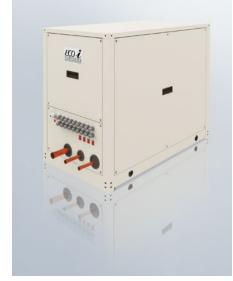
Panasonic offers a purposely engineered solution which allows for a quick and simple installation. The unit contains 5 actuating ball valves, a 30l storage vessel and PLC all housed in an IP54 rated container. Terminals on the front of the unit allow for easy wiring to the alarm terminal, high / low pressure transducers and discharge temperature sensor(s) of the condensing unit(s).
