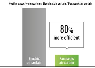
\* With the U-100PE1E5 on the PAW-20PAIRC-MS. Calculation method: Taking as consideration SCOP of the Panasonic combination of 6.0. If 100 is the energy needed for a air curtain, Panasonic Air curtain will need 1/(1-6)\*100=20.
