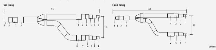
CZ-P1350BK2BM: For indoor unit side (Capacity after distribution joint is greater than 68,0kW and no more than 168,0kW).
