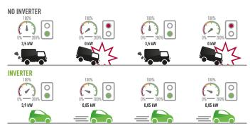
NO INVERTER Slow to start. Takes longer to reach the temperature set point. The temperature oscillates between the two extremes and never stabilises. The temperature falls and then rises quickly, leading to a consumption peak INVERTER Rapidly reaches the desired temperature. Adjusts the temperature: more comfort and greater savings, Keeps the temperature comfortable all the time
