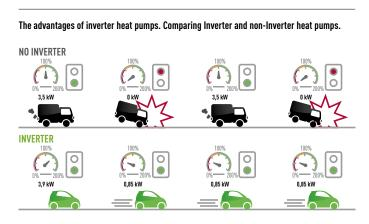
NO INVERTER Slow to start. Takes longer to reach the temperature set point. The temperature oscillates between the two extrem and never stabilises. The temperature falls and then rises quickly, leading to a consumption peak. INVERTER Rapidly reaches the desired temperature. Adjusts the temperature: more comfort and greater savings. Keeps the
