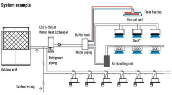
Note: The mode of running of outdoor unit depends on the Water Heat Exchanger's mode. The water pump is not included in the N2 models Water Heat Exchanger. For simultaneous operation, however, the maximum capacity is 130%. Please inquire details of this system design of Panasonic. \* Standard DX type indoor unit system.
