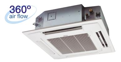
The award winning range of U1 type cassettes are smaller, shallower and lighter than previous models and feature a 950 x 950mm panel throughout. The DC-Fan motor and air discharge louvre ensure quiet, optimum air distribution.
