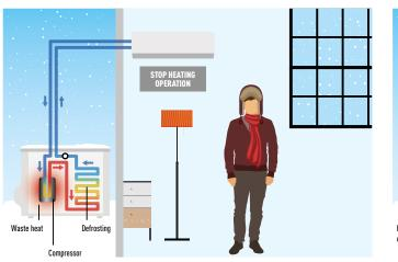
Heatcharge: The room is thoroughly warmed Defrost operation: About 5 to 6 min.
