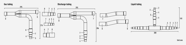
CZ-P1350PJ2BM: For outdoor unit side (Capacity after distribution joint is greater than 68,0kW and no more than 135,0kW).
