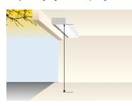
Max installation high Jet-Flow: 3,5 m Standard flow: 3,0 m
