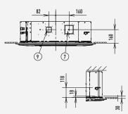
Adjust the suspension bolt length so that the gap from the lower ceiling surface becomes 30mm or more (18mm or more from the lower surface of the body) as shown in the figure. When the suspension bolt length is long, it hits the ceiling panel and installation is not possible.
