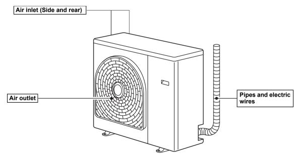
\* The image of outdoor unit in the figure is in case Model RAV-SM1403AT-E.
